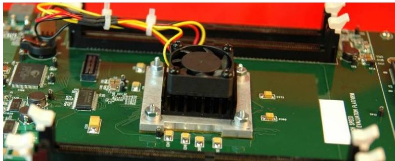
Final Heat Sink Socket Assembly With Fan Mounted On OEM Printed Circuit Board
